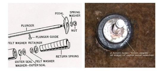
cylinder was half full at the time of doing this, however, very little if any escaped while changing seals. Replace outer seal washer lining up with drill hole and press into place. With the aid of 1/2" sockets, slot over plunger and tap outer seal washer home till it flush with master cylinder housing, replace felt washer and retainer, return spring, pedal and etc.
